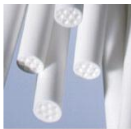
Fig. 2 Multibore ultrafiltration membrane fibers
